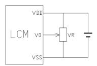
V<sub>DD~</sub>V<sub>0</sub>: LCD Driving voltage VR: 10k~20k
